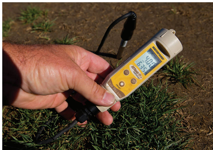
A portable EC meter is an essential tool for making decisions about leaching.
